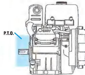
The mounting face of the P.T.O. side, MZ engine is almost flat against applications. This will make customer easier to apply their product fit against our engine compare to others.
