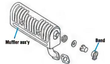
The adoption of a large muffler reduces the exhaust noise. The tail screen is also adopted to MZ125 and MZ175.
