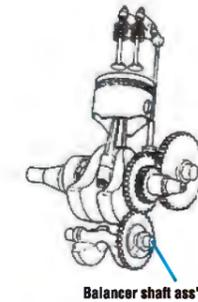
MZ engine has one balancer on 360. Big capacity single cylinder engine is able to get larger vibration. In order to cure this, balancer is needed. Balancer shape, style, and quantity depend on each company's way of thinking.
