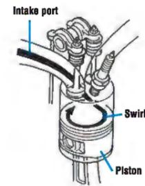
MZ engine mixture air goes into the cylinder having swirl. Mixture air needs to go into the cylinder uniformly. Also during compression and combustion, having swirl will increase the speed of plug's spark spread through the mixture air. This increases the power, fuel consumption, and cleanliness exhaust emission.
