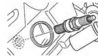
Register plug for noise reduction. Standard equipped a resistance type SPARK PLUG "BPR4ES."
