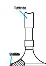
High heat resistant SUH3 steel is used. But since exhaust valve expose to more than 700 degrees Celsius instantly, at the valve face where it meets valve seat has stellite coating. Also, whole valve surface has tuftiride finish in order to increase the hardness. Together when this tuftiride finish is polished, friction of surface becomes very low which makes valve to move smoother against guides.
